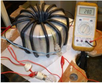
The two photographs below, show the 8kW OzInverter toroid under testing, but here it has a temporary primary cable/wire. The 8kW OzInverter has a secondary of 80 turns and a primary of 10 turns.
