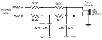
Below is a superior circuit producing quality audio with an insignificant amount of the carrier remaining. This is suitable for a more sophisticated HiFi amplifier/speaker configuration. The output is good for 10Hz to 15KHz at about 3V peak to peak (1V RMS) at 1KHz.
