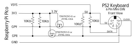
The recommended MOSFET is a TN0702N3-G or ZVNL110A however the commonly available 2N7000 has been tested and works well.
