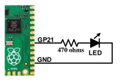
When you have saved and run this program you should be greeted by the LED flashing on and off. It is not a great program but it does illustrate how the PicoMite firmware can interface to the physical world via your programming.
