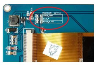
pads marked "1963-PWM". The brightness can then be set using the BACKLIGHT command via the SSD1963 controller (this is automatic, nothing needs to be configured).
