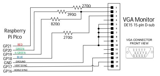
The output is in the standard VGA format with a pixel rate of 25.175MHz and a frame rate of 60Hz.
