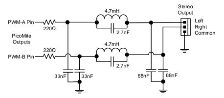
Both circuits are designed to feed an amplifier (not directly drive a headphone or speaker) and rely on capacitor coupling into the following amplifier (most have this).
