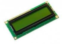
d4, d5, d6 and d7 are the numbers of the I/O pins that connect to inputs D4, D5, D6 and D7 on the LCD module (inputs D0 to D3 and R/W on the module should be connected to ground). 'rs' is the pin connected to the register select input on the module (sometimes called CMD or DAT). 'en' is the pin connected to the enable or chip select input on the module.
