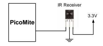
Vishay TSOP4838, Jaycar ZD1952 and Altronics Z1611A. Note that the I/O pins on the Raspberry Pi Pico are only 3.3V tolerant and so the receiver must be powered by a maximum of 3.3V. The Raspberry Pi Pico 2 is different and can withstand 5V.
