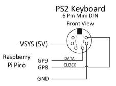
The I/O pins on the RP2350 series of microcontrollers can withstand 5V (while powered up) so the keyboard can be directly connected as illustrated with the 5V supplied by the VSYS pin on the Raspberry Pi Pico 2. The keyboard is enabled with the OPTION KEYBOARD command.
