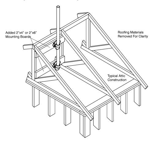
Mounting Through a Roof or Roof Overhang
