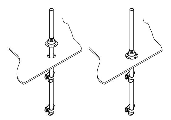
Seal the layers of roofing material to each other with a silicone caulk or sealant so that moisture is prevented from penetrating through to the wood. Apply a generous amount of sealant to the base of the seal. Slide the seal the rest of the way down onto the roof and locate it so that the base is centered over the hole. Southwest Windpower
