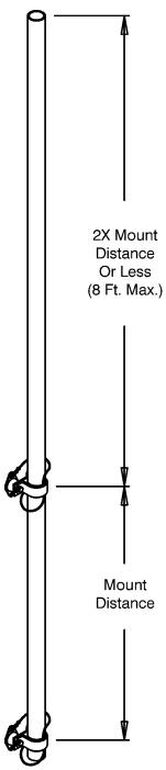
In all cases the system should be mounted as solidly as possible to the most rigid part of the structure.
