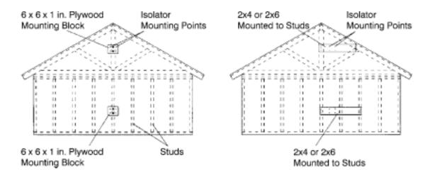
If only a single wall stud is available for mounting, plywood blocks at least  $\frac{3}{4}$ " (19 mm) thick and 6" (150 mm) square should be centered on the stud and mounted with 3" (75mm) long lag bolts and washers. The mounts should be centered on these blocks.
