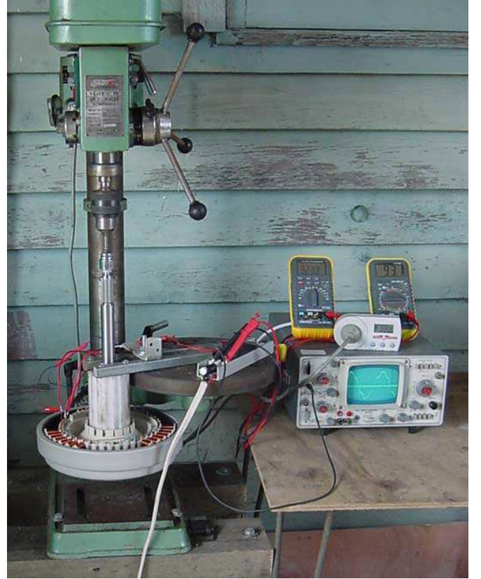
Fig 5. Experimental rig for efficiency measurement. The bench drill drives the alternator shaft. Electrical power consumption of the drill motor is measured by Sparometer, a white instrument between voltmeters. Note the removed poles of the alternator stator.
